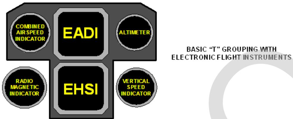
BASIC "T" GROUPING WITH ELECTRONIC FLIGHT INSTRUMENTS
